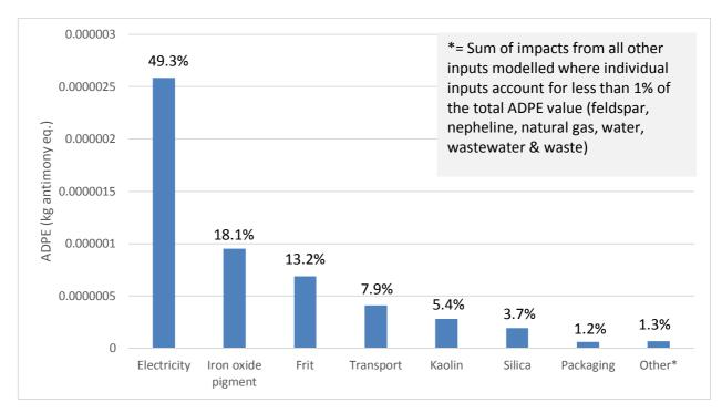
Figure 8: ADPE (kg antimony eq.) per kg of Lapitec sintered stone slab production
