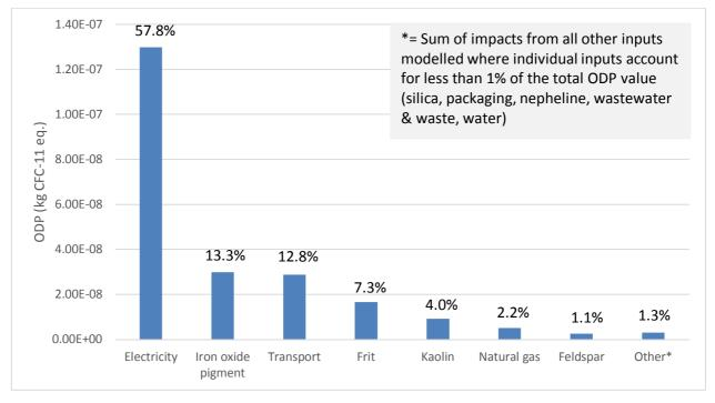
Figure 4: ODP (kg CFC-11 eq.) per kg of Lapitec sintered stone slab production
