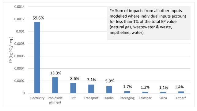
**Figure 6**: EP (kg PO<sub>4</sub><sup>3-</sup> eq.) per kg of Lapitec sintered stone slab production
